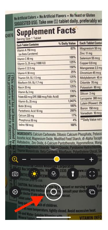
The buttons on the bottom let you control which camera you are using, the brightness, apply filters, turn on the flashlight, detect objects and the target button at the bottom captures a screenshot.
